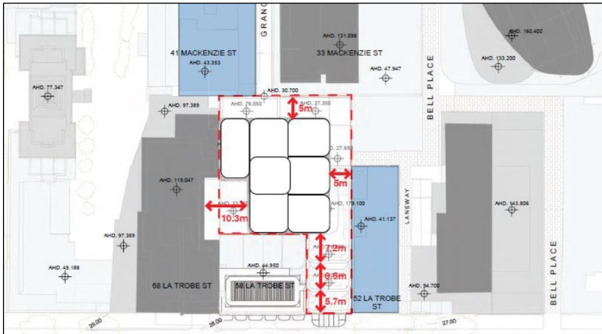
Figure 10 – extract of the Town Planning Report depicting the proposed tower setbacks prepared by Urbis dated October 2024 (Rev. 02)
